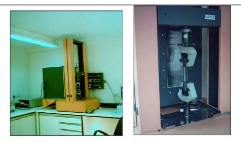
Figure 18 Lloyd Instruments. Testing facilities of mechanical properties test for rectangular speciments(3-5 mm and 20mm ±10%)
