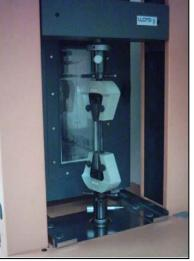
Figure 2 Lloyd Instruments. Testing facilities of mechanical properties test for rectangular speciments(3-5 mm and 20mm ±10%)
