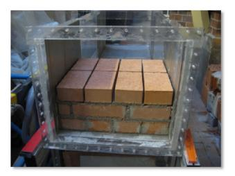
Fig. 12: Composite wall construction; single shell masonry of traditional solid bricks during the construction phase.
