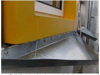
Fig. 4: Aluminium plates to measure the leakage
