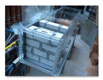
Fig. 24: Water tank with two wall test arrangements that are under construction in-situ. In front: the double shell masonry of sand-lime bricks with heat insulation and air gap. In the background: the single shell masonry of hollow bricks with external heat insulation and ventilated curtain façade.
