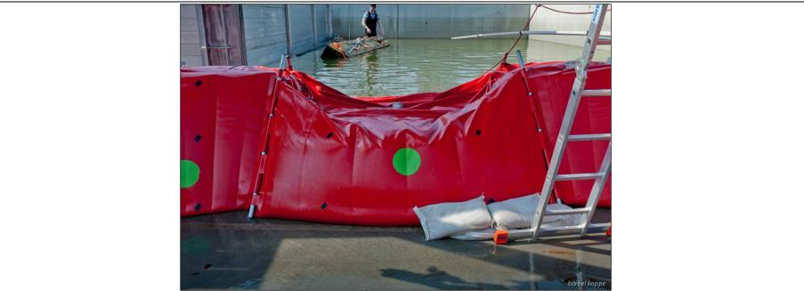
Fig. 8: Straight product configuration of the system DADLER in the testing facility of the TUHH in Hamburg-Wilhelmsburg<sup>14</sup>
