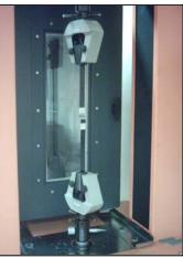
Figure 17 Lloyd Instruments . Test facility of adhesion test for rectangular speciments(wide:25mm ± 5% and long: 100mm±5%) Velocity of test: 3 mm min-1
