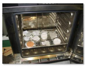
Figure 18: Building material test samples in the drying oven to determine their oven-dry mass.
