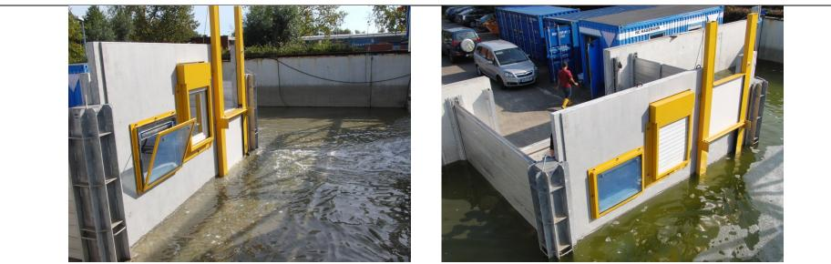
Fig. 1: Door, window and basement window barriers
