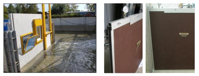
Figure 35: Aquastop system – Door, window and Figure 36: Collad'eau basement window barriers
