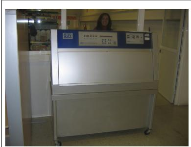
Figure 10: Resistance to UV radiation in presence of moisture. Ref: Sika
