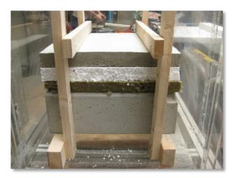
Fig. 18: Cross section of the tested composite floor construction; bottom-up: reinforced concrete floor, footstep sound and heat insulation, cement screed, carpet. The timber frame prevents the floating of constituents.
