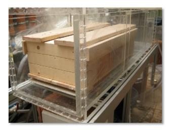
Fig. 16: Suspended timber floor; test arrangement consisting of structural joists, heat and sound insulation, plasterboard ceiling, and covering floor
